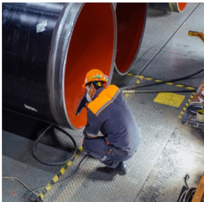
Moreover, aligned glass flake fillers in **HEGGEL Flake 710** are impermeable barriers and in turn effective in withstanding high medium temperatures.
